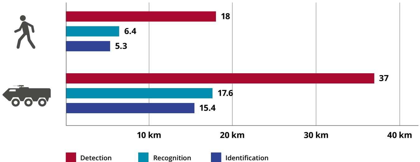
Conditions for SSIP CAM program: Contrast 30%, Over cast daylight, Sky ratio 3, Visibility 80km, 50% probability, NFOV 0,4° (H), Dimensions Man: 0.45m × 1.7m. Vehicle dimensions NATO target 2.3m × 2.3m
